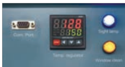
Electronic over temperature shutdown system.
